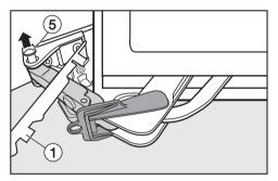
■ Push hinge pin ⑤ up and out from underneath.
